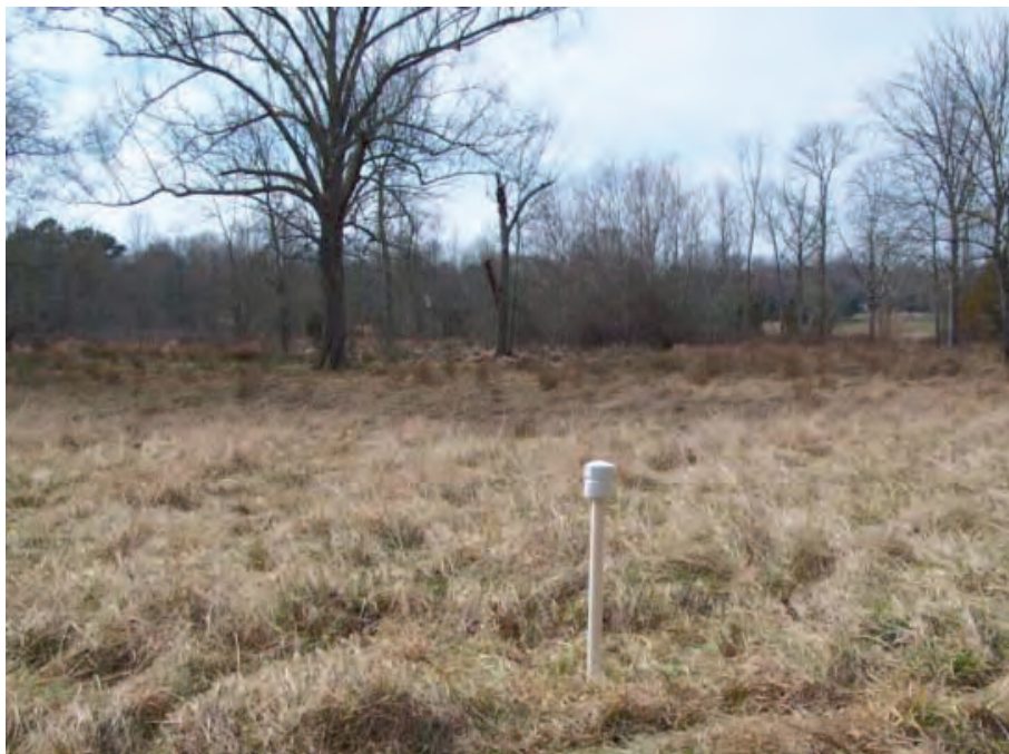
Figure 15. Sixmile Creek Site monitoring well.
