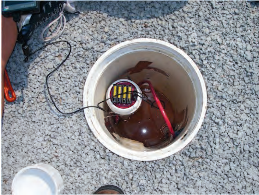
Figure 4. Monitoring well in porous concrete parking lot
