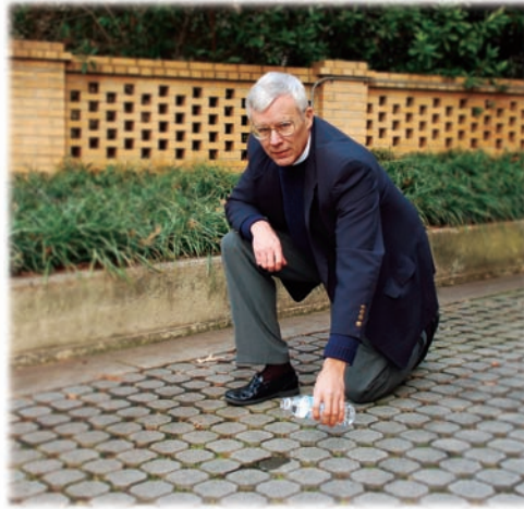
Ferguson, armed with his water bottle, can perform on-the-spot tests of the porosity of paved surfaces.
